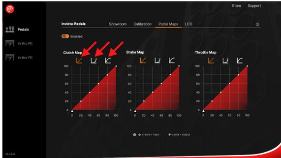
As we briefly mentioned, a real race car will not have a linear throttle response. An example will be an Audi R8 LMS GT3, which has less activation of the throttle at the beginning of the pedal activation, increasing as you progress through the travel. Similarly, you can adjust your curves based on your driving conditions—all in search of ultimate performance.
