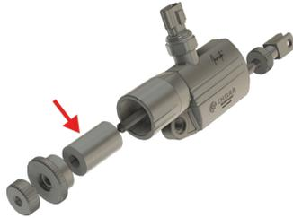
6. Grab the small thumbnut and turn it onto the shaft clockwise until it locks the larger thumbnut in place.
