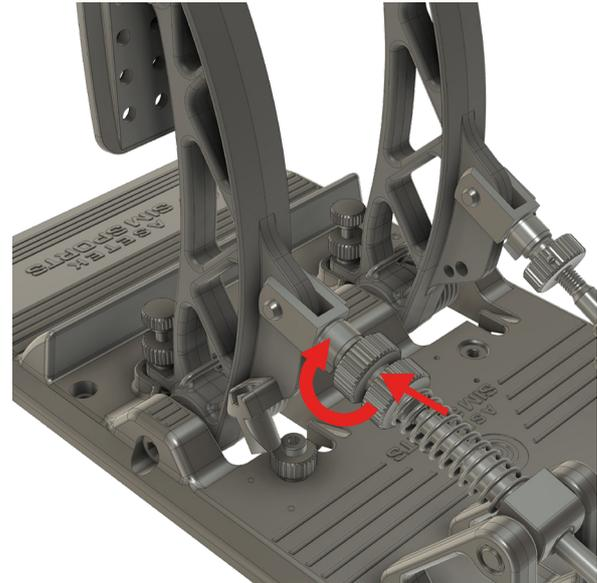
2. Adjust preload on the spring by turning the bottom thumbnut (in contact with the spring):
