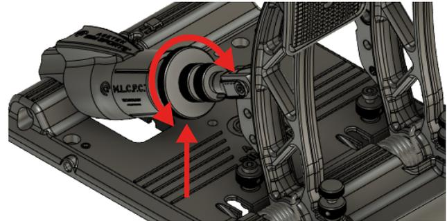
3. Re-tighten the thumbnut and rotate clockwise, while holding the piston firm, until it locks up against the piston.
