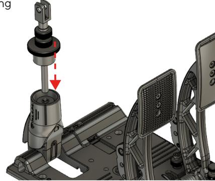
8. Re-insert the clevis lock pin.
