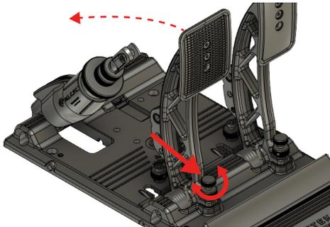
7. Adjust the pushrod length by turning the clevis until it approximately matches up with the hole in the pedal arm. Re-insert the clevis lock pin.
