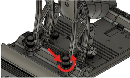
2. Push the pedal slightly forward and rotate the thumbscrew (Clockwise to move the pedal forwards, Counter-Clockwise to move the pedal backwards)
