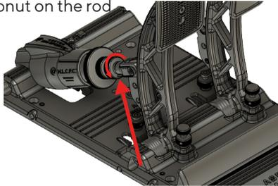
2. Remove the clevis lock pin
