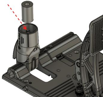
7. Grab the rod and carefully insert into the elastomer and over the spring
