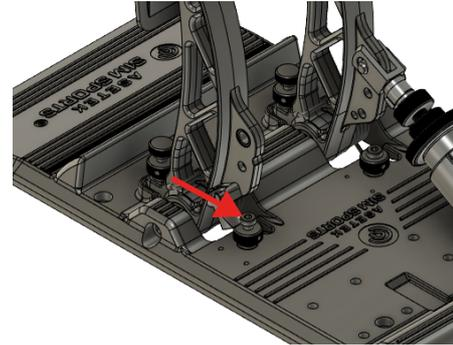
3. Re-tighten the thumbnut by rotating it clockwise.
