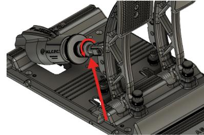
2. Remove the clevis lock pin.
