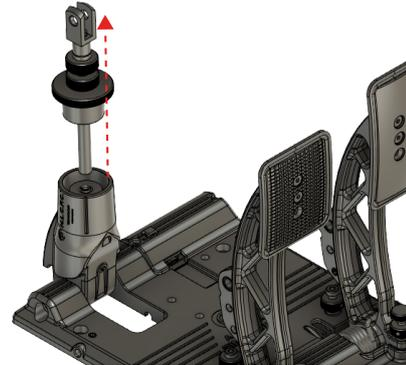
5. Carefully remove the elastomer with your fingers. If you cannot get it out with your fingers, use the pushrod spring to pull it out.
