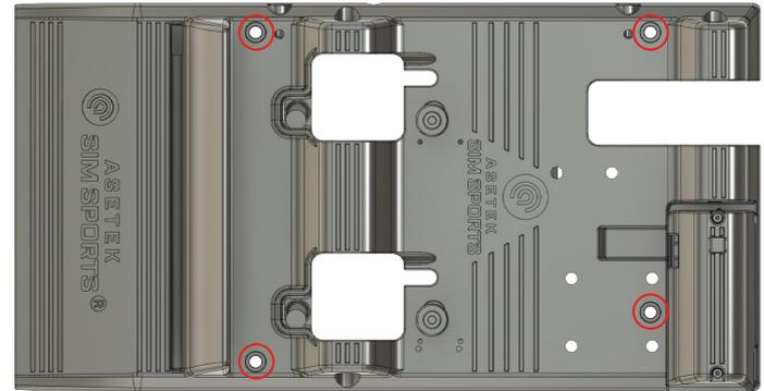
The baseplate is designed to be used with M6 screws, and holes in your rig should be with  $\text{Ø}6,4$  diameter. It is also compatible with the included M6 slot nuts.
