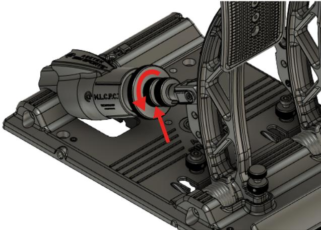
2. Rotate the piston to adjust the amount of preload on your brake:
