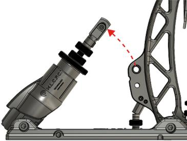
4. Carefully remove the rod out of the brake cylinder
