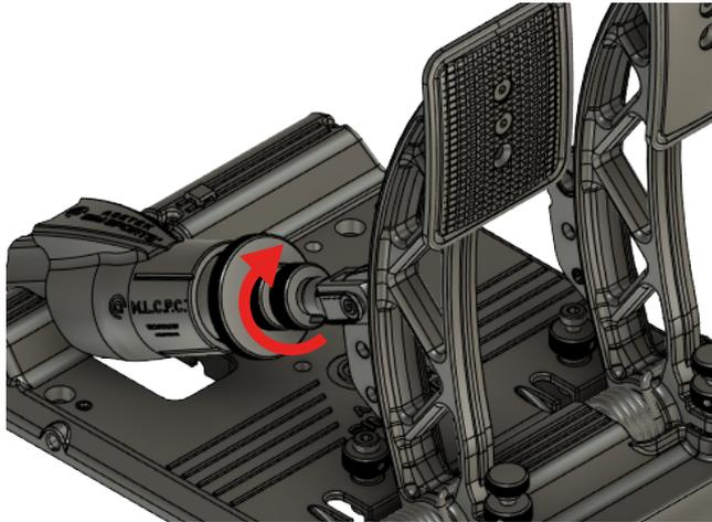
2. Remove the clevis lock pin
