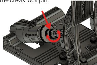
Because of the built-in spring in the pushrod, there will be a small preload requiring you to most likely having to pull back the clevis a bit while inserting the lock pin. This is normal.
