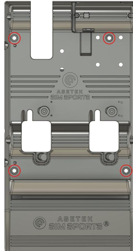
4. Mount the pedals to the existing holes using the four (4) provided M6x20 screws, four (4) washers, and four (4) nuts or four (4) M6 slot nuts (depending on your rig).
